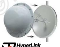
HyperGain® Radome Covers are an ideal way to provide additional protection to our parabolic dish antennas. These light weight radome kits feature fiberglass construction and UV stable gray finish. Drain holes are provided on the radome cover to help prevent moisture build-up inside the dish antenna.
